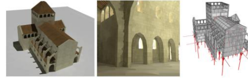
Figure 1: Our method generates models of masonry buildings that are structurally stable. In this building based on Clery Abbey in France, parameters controlling the flying buttresses, columns, and window sizes have been automatically optimized to support a stone vaulted ceiling. The right image shows reaction forces at the ground plane. We solve for forces at all block interfaces, and apply a compression-only constraint for masonry materials.
